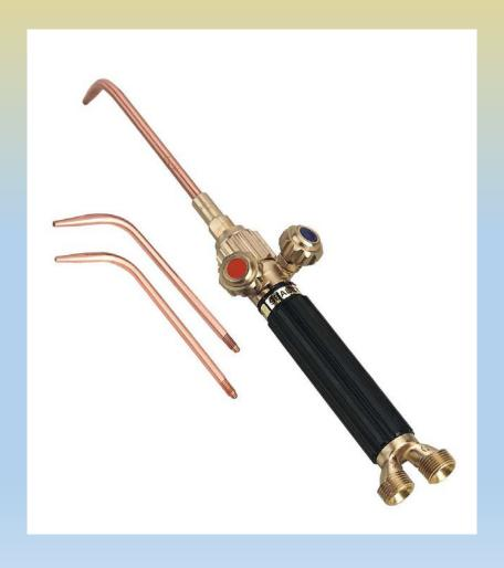
A welding torch has two control valves (oxygen and fuel) and one hole in the tip of the torch. Tip sizes vary depending on the hole diameter.
