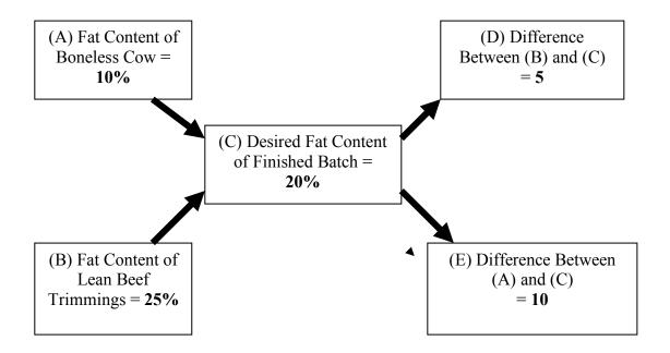
The difference in A and B = 15 and the sum of D and E = 15 so the Pearson Square is set up properly.
