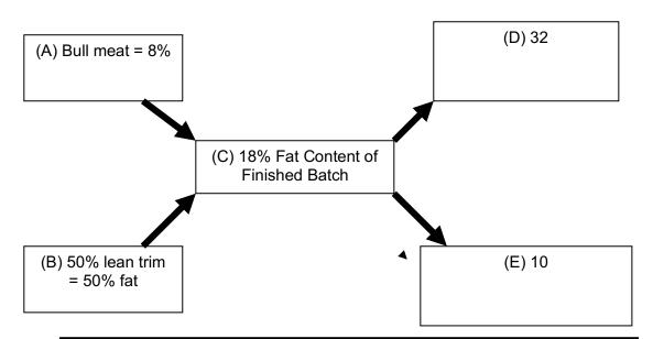
The difference in A and B = 42 and the sum of D and E = 42 so the Pearson Square is set up properly.
