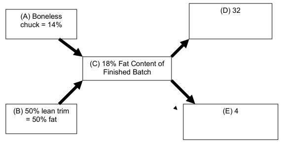
The difference in A and B = 36 and the sum of D and E = 36 so the Pearson Square is set up properly.
